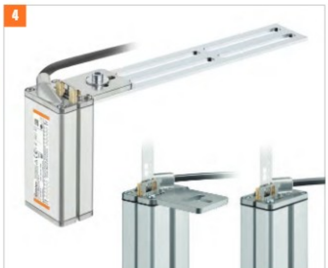
4 Maximum flexibility: Connect sensor to the car mounting and adjust optimally (three possible mounting types in 90° steps). Maximum compactness: Whether with mounting plate or T-slot, the system is suitable for the narrowest installation spaces.
