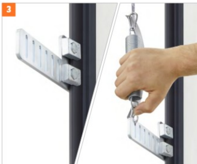
3 At the shaft pit: Fit the rail mounting. Hook the tension spring and securing band into the snap nook and connect to the rail mounting (same slot as in shaft head). Cut coded band to length and use the snap hook to connect it to the tension spring and securing band.
