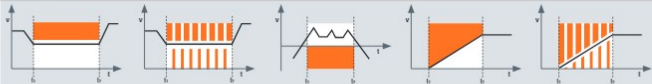
SLS – Safely-Limited Speed SSR – Safe Speed Range SDI – Safe Direction SLA – Safely-Limited Acceleration SAR – Safe Acceleration Range
